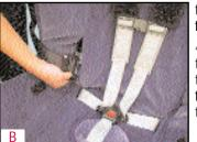
3 Pull the vehicle belt out and pass it through the first belt slot, from the front of the restraint to the rear (*Fig B*).
